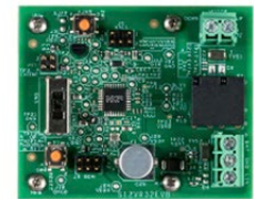
S12VR32EVB Relay-based DC S12VR32 evaluation board
