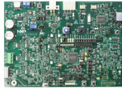
S12ZVMC256EVB 3-phase BLDC and PMSMS12ZVMC256 evaluation board
