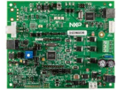
S12ZVM32EVB 3-phase BLDC and PMSM S12ZVM32 evaluation board
