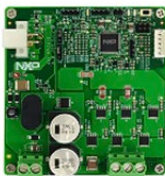
S12ZVM-EFP Electrical Fuel Pump S12ZVML128 reference design
