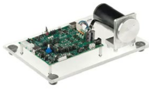
MTRCKTSBNZVM128 3-phase BLDC Motor control kit
