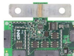
RD9Z1-638BJBEVM Battery junction box MM912J638 reference design
