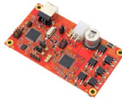
S12ZVML-MINIXXX 3-phase PMSM Motor control kit
