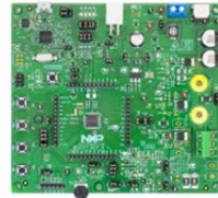
S12ZVMAEVB Unidirectional DC S12ZVMA evaluation board
