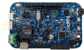
DEVKIT-S12VR64 Relay-based DC S12VR64 evaluation board
