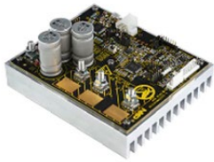
MCSXSR1CS12ZVM 3-phase BLDC and PMSM S12ZVML128 High-current evaluation board
