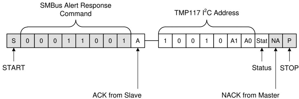
**Figure 7-11. SMBus ALERT Timing Diagram**
