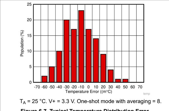
$T_A = 25^\circ\text{C}$ ,  $V_+ = 3.3\text{ V}$ . One-shot mode with averaging = 8.
