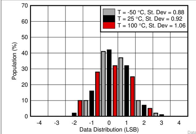
**Figure 6-6. Data Reading Distribution Over Temperature (No Averaging,  $V_+ = 3.3\text{ V}$ )**
