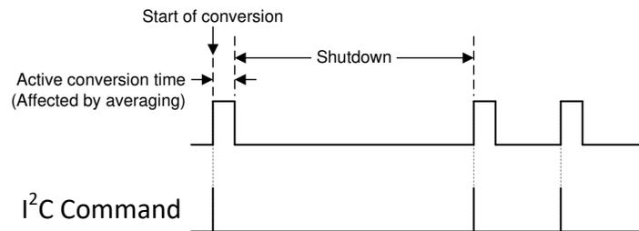
**Figure 7-4. One-Shot Timing Diagram With AVG[1:0] = 00**
