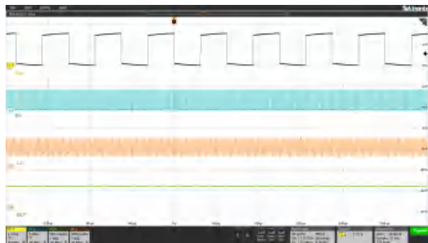
Figure 8-34. LED Analog Dimming at 50% Duty Cycle and 20 kHz
