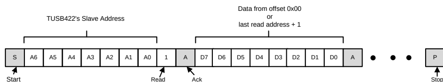
图 7. I2C Read Without Repeated Start
