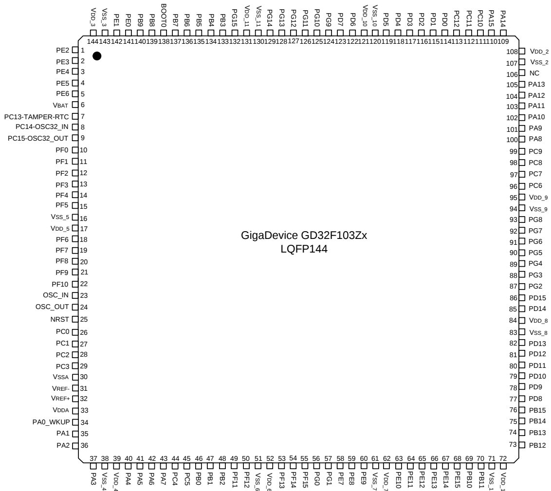
Figure 3. GD32F103Zx LQFP144 pinouts
