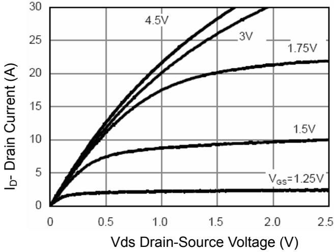
**Figure 1 Output Characteristics**
