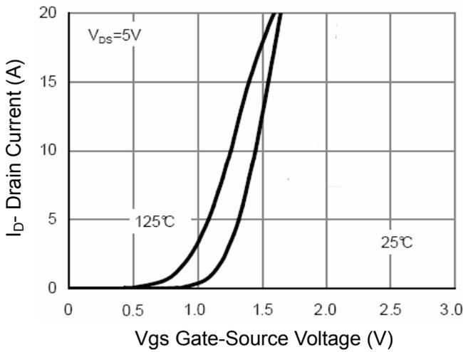
**Figure 2 Transfer Characteristics**
