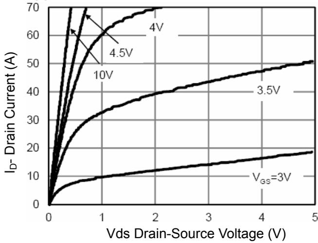
Figure 1 Output Characteristics
