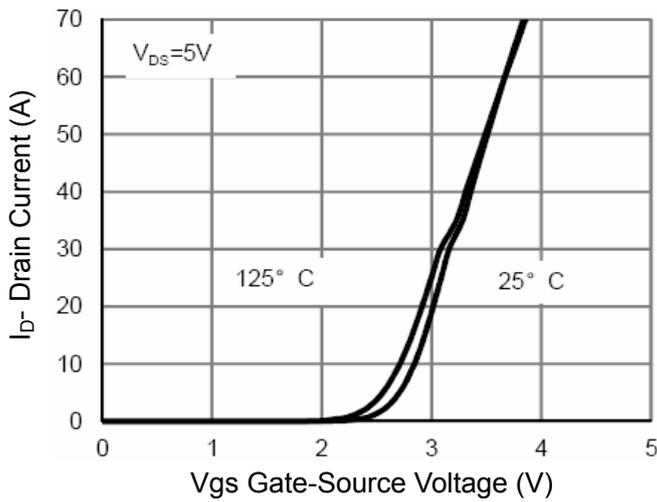
Figure 2 Transfer Characteristics
