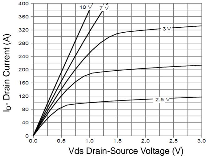
Figure 1 Output Characteristics
