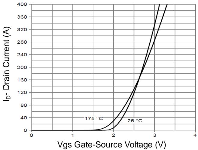
Figure 2 Transfer Characteristics
