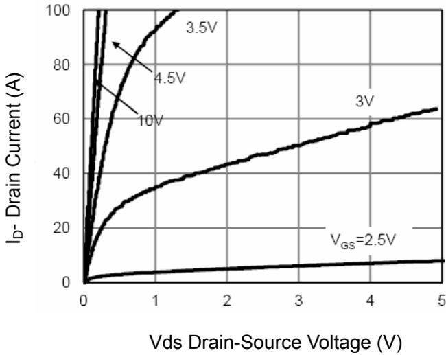
Figure 1 Output Characteristics
