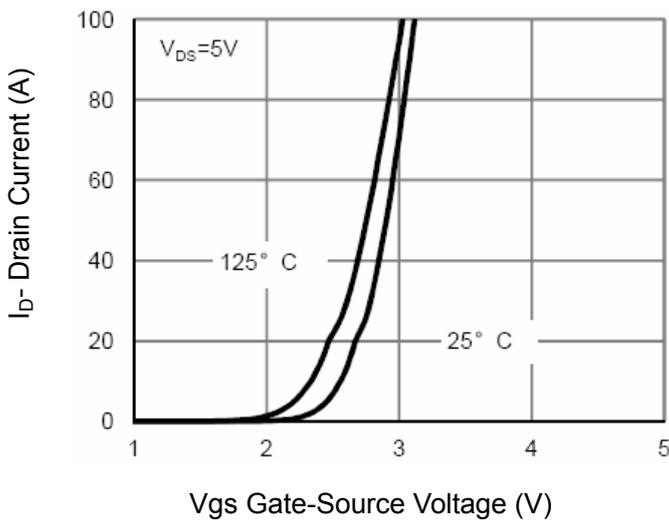
Figure 2 Transfer Characteristics
