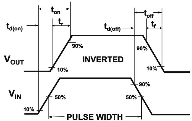
Figure 2: Switching Waveforms
