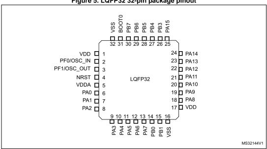
Figure 5. LQFP32 32-pin package pinout
