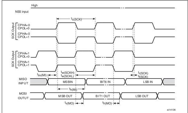
Figure 25. SPI timing diagram - master mode
