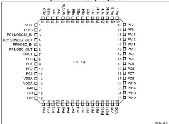
Figure 3. LQFP64 64-pin package pinout
