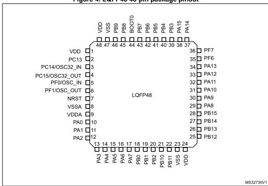
Figure 4. LQFP48 48-pin package pinout
