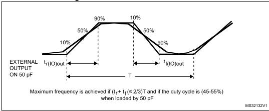
Figure 18. I/O AC characteristics definition
