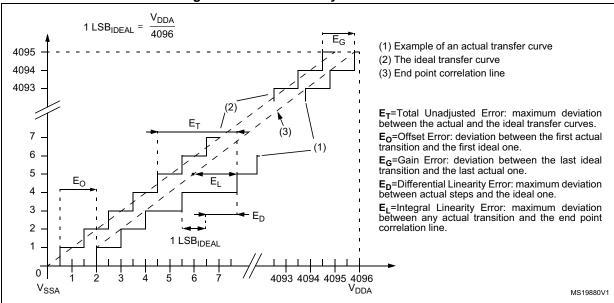
Figure 20. ADC accuracy characteristics
