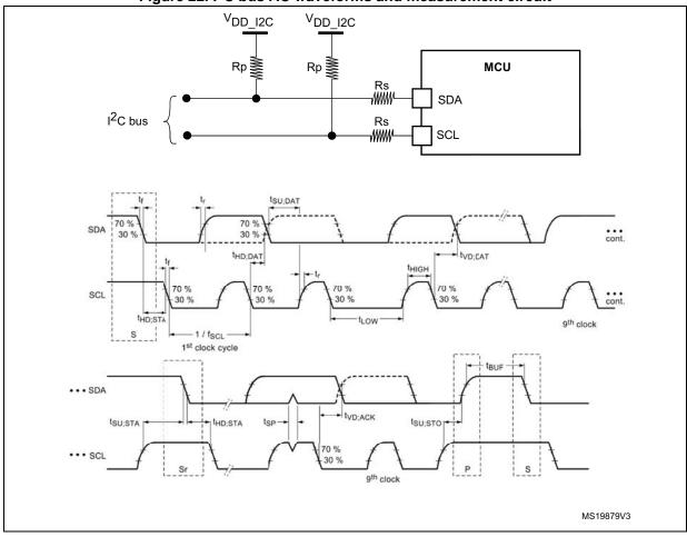
Legend: Rs: Series protection resistors. Rp: Pull-up resistors. V<sub>DD 12C</sub>: 1<sup>2</sup>C bus supply.
