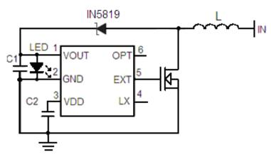
Figure1 without expending output current MOSFET's application (one or two dry batteries)
