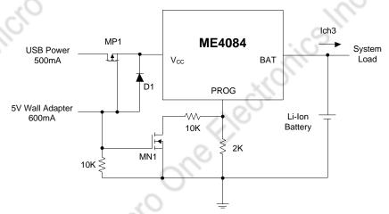
Fig.5: Combining Wall Adapter and USB Power
