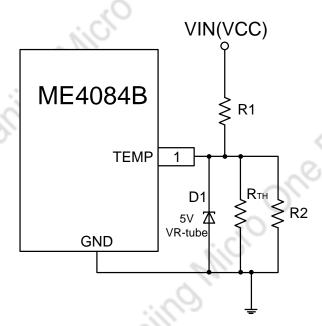
The values of R1 and R2 in the application circuit can be determined according to the assumed temperature monitor range and thermistor's values. The Follows is an example: Assume temperature monitor range is TL~TH, (TL<TH); the thermistor in battery has negative temperature coefficient (NTC, RTL is thermistor's resistance at
